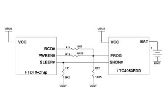
FT-X enables optimal battery charging!
