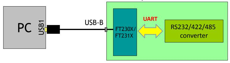
Integrate UART interface into embedded system application
